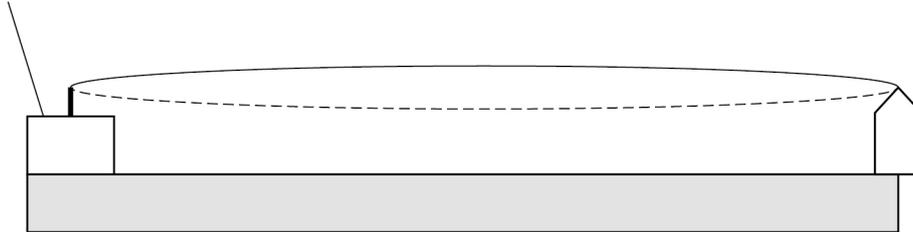
The string in **Figure 13** is replaced with one that has 9 times the mass per unit length of the original string. All other conditions are kept constant, including the frequency of the vibration generator and the tension in the string.
