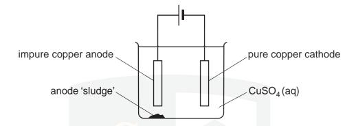
The impure copper anode contains small quantities of metallic nickel, zinc and silver, together with inert oxides and carbon resulting from the initial reduction of the copper ore with coke. The copper goes into solution at the anode, but the silver remains as the metal and falls to the bottom as part of the anode 'sludge'. The zinc also dissolves.
