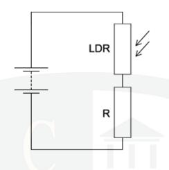
The resistance of the LDR is equal to the resistance of *R* when no light falls on the LDR. When the light intensity falling on the LDR increases, which statement is correct?
