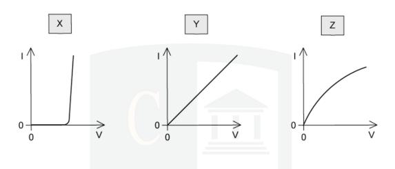
The components are a metal wire at constant temperature, a semiconductor diode and a filament lamp.
