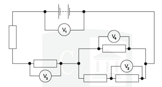
The reading on voltmeter  $V_1$  is 8.0 V and the reading on voltmeter  $V_2$  is 1.0 V. What are the readings on the other voltmeters?
