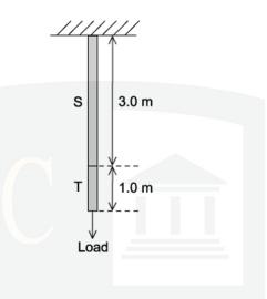
When a load was hung from the wires S stretched by 1.5 mm and T by 1.0 mm.
