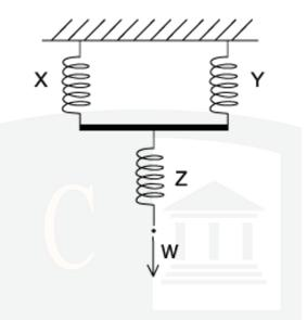
Springs X and Y are identical and have a spring constant k. Spring Z has a spring constant of 3k.
