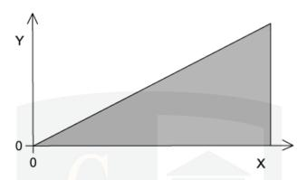
The area under the graph shows the total strain energy stored in the wire when stretched.
