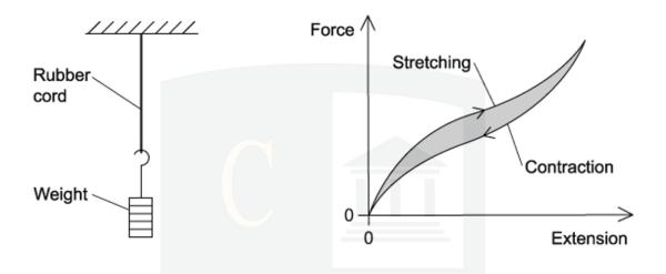
The graph shows the force-extension curve for contraction (below) and the force-extension curve for stretching.
