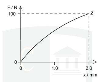
What could be the value of the strain energy stored in the wire when it is stretched elastically to point Z?
