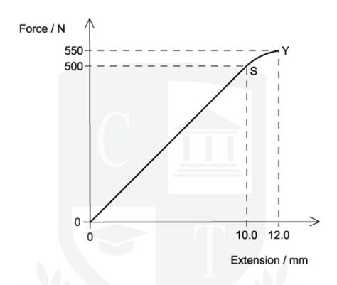
When the sample was stretched from 0 to 12.0 mm extension, what is the work done? Assume that the curve SY is a straight line to simplify the calculation
