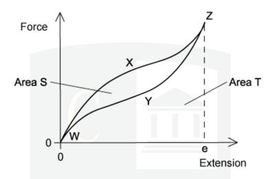
As the force is increased, the curve follows the path WXZ to extension x. As the force is reduced, the curve follows the path ZYW to return to zero extension.
