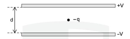
The separation of the plates is d. The droplet is observed to be stationary when the upper plate is at potential +V and the lower plate is at potential -V.
