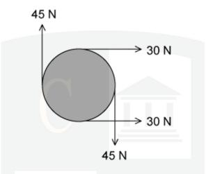
Which of the following describes the resultant force and resultant torque on the object?
