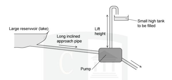
In one such pump the long approach pipe holds 500 kg of water. A valve shuts when the speed of this water reaches  $2.0 \text{ m s}^{-1}$  and the kinetic energy of this water is used to lift a small quantity of water by a height of 15 m.
