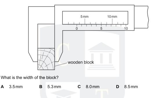
45 The width of a wooden block is measured using vernier calipers.
