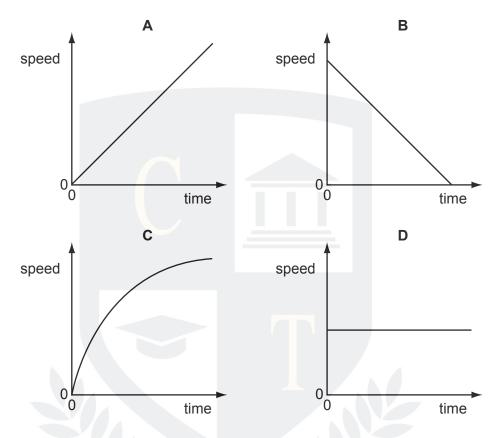
38 Which speed-time graph shows an object moving with non-uniform acceleration?
