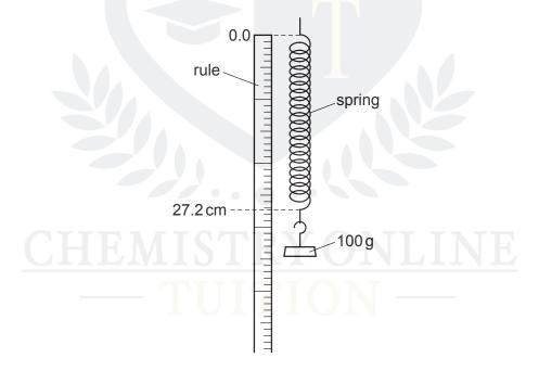
The 100 g mass is replaced with a 600 g mass. The length of the spring is now 89.7 cm. The spring has not reached the limit of proportionality.
