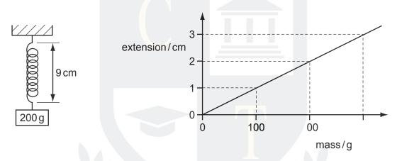
The 200 g mass is replaced with a 100 g mass. What is the new length of the spring?
