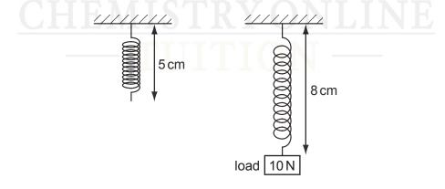
The 10 N load is replaced by a 20 N load. What is the new length of the spring?
