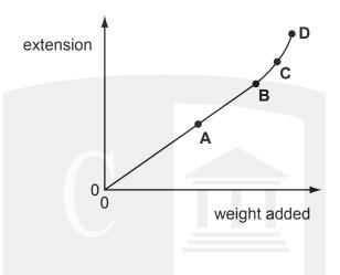
**1**5 Which part of the graph shows the limit of proportionality for an elastic solid?
