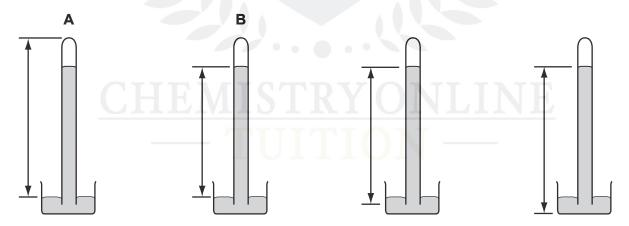
52 A water manometer is connected to a gas supply. The diagram shows the water levels.
