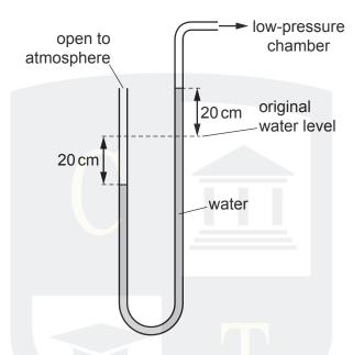
When one end of the manometer is connected to a low-pressure chamber, both water levels in the manometer change by 20 cm. The gravitational field strength g is 10 N/kg.
