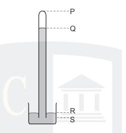
The mercury level in the tube falls, leaving a vacuum at the top.
