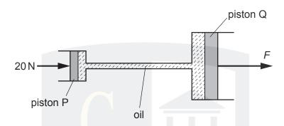
Piston P has an area of 5.0 cm<sup>2</sup> and piston Q has an area of 25 cm<sup>2</sup>.
