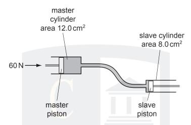
The cross-sectional area of the master cylinder is  $12.0 \text{ cm}^2$  and the cross-sectional area of the slave cylinder is  $8.0 \text{ cm}^2$ . The force applied to the master piston is 60 N, producing a pressure of  $5.0 \text{ N/cm}^2$ .
