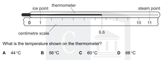
9 A liquid-in-glass thermometer contains mercury.
