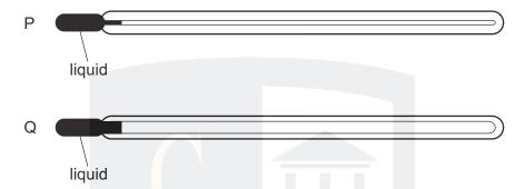
The thermometers are identical except that Q has a capillary tube with a larger internal diameter than P.
