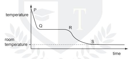
In which part of the curve is latent heat released?
