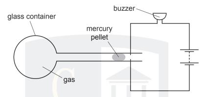
The mercury pellet moves and completes the circuit.
