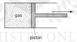
The piston is moved so that the volume occupied by the gas increases. The temperature remains constant.
