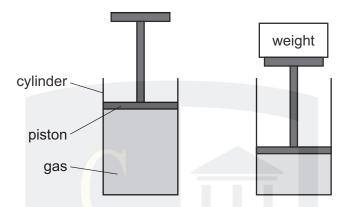
A weight is put on the piston. The volume of gas supporting the piston decreases but the temperature of the gas is unchanged.
