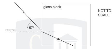
What is the angle of refraction in the glass and what is the critical angle?
