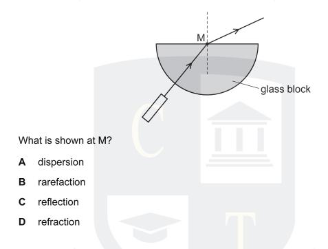
**2**<sup>7</sup> A ray of red light from a laser passes into a semi-circular glass block.
