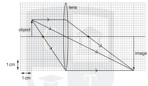
The arrangement is shown on the full-scale ray diagram.
