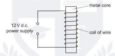
The core becomes a magnet when the current is switched on. It remains a magnet after the current is switched off.
