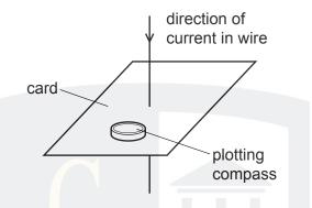
A plotting compass is placed on the card.
