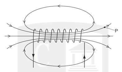
What is the effect on the magnetic field at the point P of using a larger current in the opposite direction?
