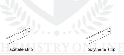
Two rods **X** and **Y** are brought up in turn to these two strips. Rod **X** attracts the acetate strip but repels the polythene strip. Rod **Y** does not repel either the acetate strip or the polythene strip.
