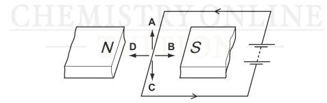
20 A simple d.c. motor consists of a coil that rotates between the poles of a permanent magnet. The turning effect is increased by winding the coil on a metal cylinder.
