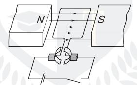
The switch is closed and the coil rotates.
