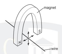
The current in the wire can be reversed. The poles of the magnet can also be changed over.
