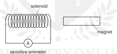
The magnet is pushed towards the solenoid. It accelerates, then moves at constant speed, then decelerates and stops inside the solenoid.
