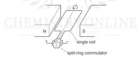
The split-ring commutator reverses the current in the coil as the coil rotates.
