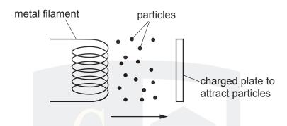
The particles are attracted by a charged plate.
