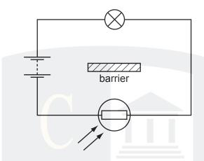
When low intensity light falls on the LDR, the lamp glows dimly.
