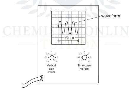
What is the time taken for one cycle of the waveform?
