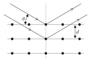
(i) Show that the extra distance travelled by the electron beam reflecting off the second layer of atoms is given by  $2d\sin\theta$ .
