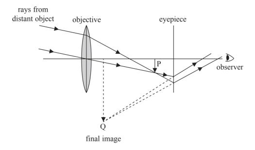
The objective produces an image at P. This image becomes the object of the eyepiece, which produces a final image at Q.
