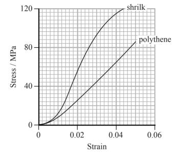
(a) (i) Calculate the force applied to the shrilk at a strain of 0.02 cross-sectional area =  $1.2 \times 10^{-6}$  m<sup>2</sup>
