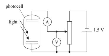
(i) Explain how the potential divider circuit can produce a range of values from 0 to 1.5 V on the voltmeter.
