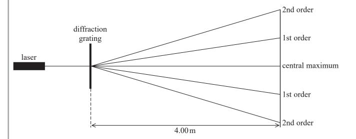
The student measured the distance between the central and a 2nd order maximum as 1350 mm. The diffraction grating had 300 slits mm<sup>-1</sup>.
