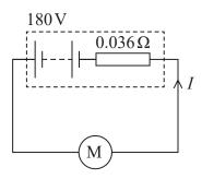
The motor has a maximum power of 88 kW.
