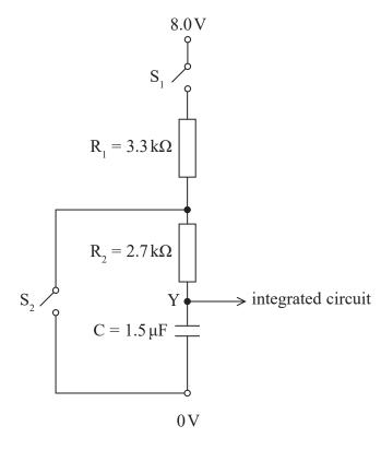
(a) Initially the capacitor is uncharged. The switch  $\mathbf{S}_1$  is closed.
